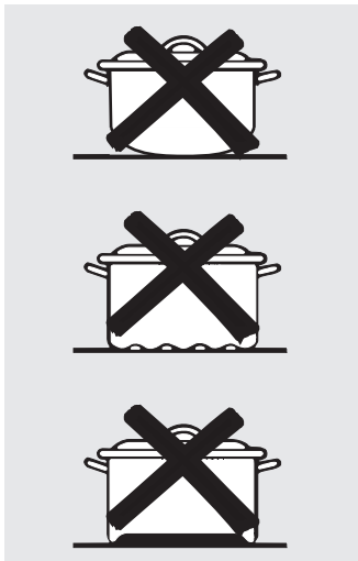
Pans with rounded, curved, ridged or warped bottoms are not recommended.
