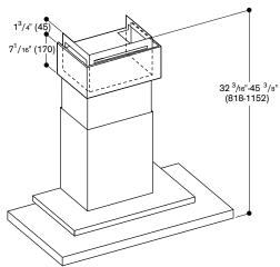
\* Suitable for ceiling heights of 8 ft. (2.45 m) to 9 ft. (2.75 m); Specifications refer to a distance from floor to lower duct cover edge of 5.2 ft. (1.60 m).
