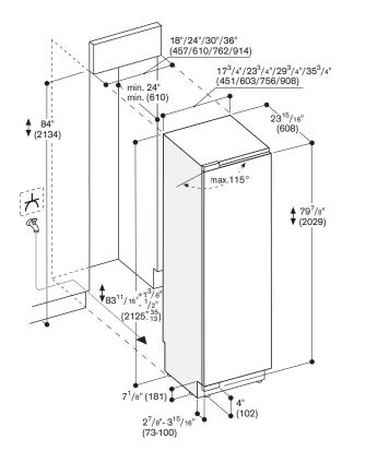
The door face dimensions are designed for a maximum gap of 1/6" (3 mm). \* For a flush-mounted appearance, the minimum cut-out depth must be 25". See more details on pages 223 and 225.
