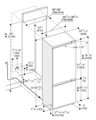
The door face dimensions are designed for a maximum gap of 1/8" (3 mm).
