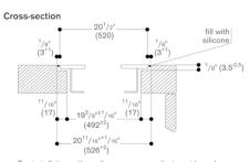
For installation with appliance cover or adjustment bar, observe the deeper notch and the slot width front and back.
