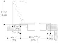
Installation with appliance cover/adjustment strip; Flush Installation
