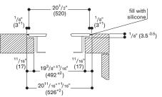
When installating with appliance cover or adjustment strip, pay attention to the deeper cut-out and the front and rear groove width.
