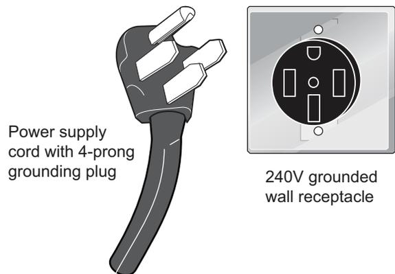
**Figure 1: Grounding plug and receptacle**
