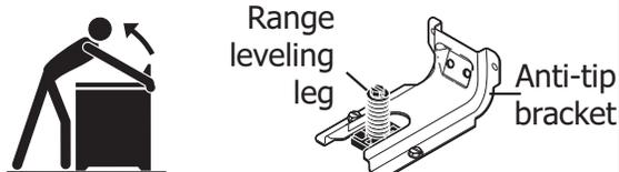
To check if the anti-tip bracket is installed properly, use both arms to grasp the rear edge of the range back. Carefully attempt to tilt range forward. When properly installed, the range should not tilt forward.
