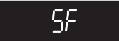
Figure 34: Display showing Sabbath failure
