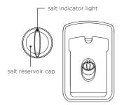
The salt reservoir is located on the inside of the drawer next to the detergent dispenser. It holds up to approximately 0.8lb (350g) of salt (actual capacity will vary depending on brand and grain size of salt used).
