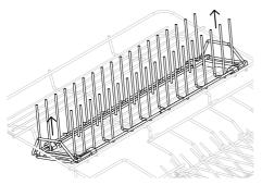
Grip the front and back handles and pull up to unclip.
