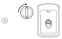
Refit the cap, turning clockwise until secure.
