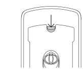
Press the latch down to open the dispenser. Check that the dispenser is empty and dry.
