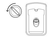
Turn the cap anticlockwise and remove.
