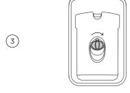
Refit the plug, turning clockwise until secure.
