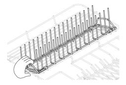
Slide the tines backward or forward by pushing or pulling the front handle.
