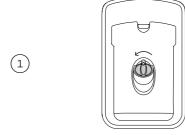
Turn the plug anticlockwise and remove.
