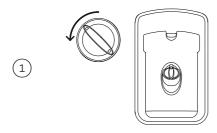
Turn the cap anticlockwise and remove.
