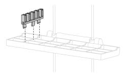
This clips onto the adjustable racks and supports knives and other utensils during the wash.
