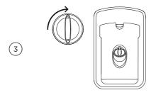
Refit the cap, turning clockwise until secure. If you are not washing your dishes immediately after filling the salt reservior, we recommend running a RINSE cycle to remove any salt water or spilt granules.
