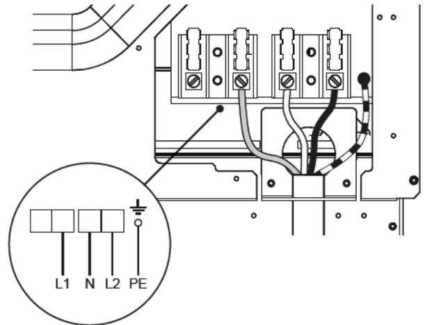
**3-Wire Connection (using supplied Ground lead)**
