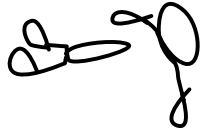
Wire clip (2) (for securing Drain hose joiner)
