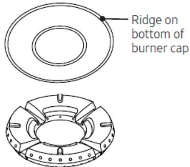
1. Place the burner heads as shown. The locator tab on the head goes in the keyed hole as shown.
