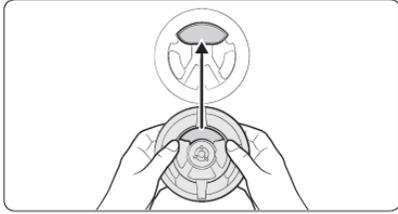
1. Orient the burner head so the opening for the electrode aligns with the electrode.
