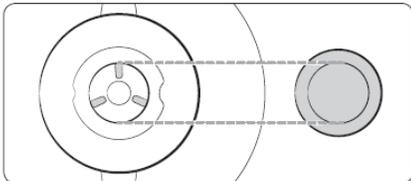
3. Size the burner caps to the burners, then install the caps on the heads.
