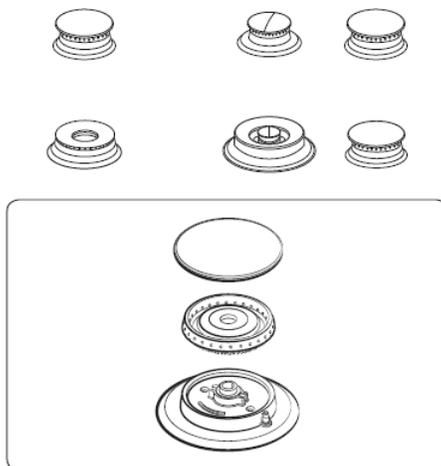
1. Place the burner heads on their bases (see left). The electrodes fit in the slot in the bottom of the heads, which should lie flat.
