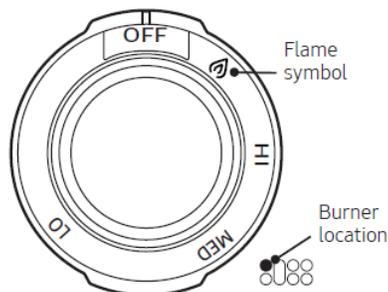
1. Push-turn a burner knob to the flame symbol. (A “clicking” sound means the electronic ignition system is functional. The burner ignites about 4 seconds later, after air is purged from the line.)
