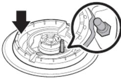
2. Install the burner head so the electrode passes through its opening in the head. Ensure the burner head lies flat on the stove top.
