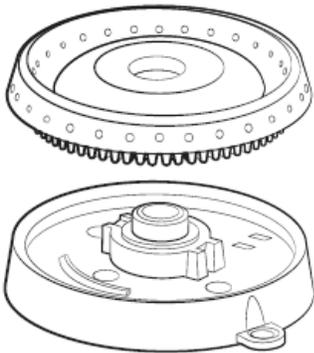
1. Put the burner heads on the burner bases. The bottom of the head fits within the burner base.
