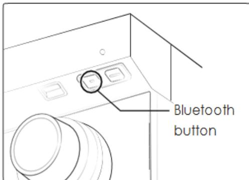
The Bluetooth button is under the rangetop front lip on the right-hand side.
