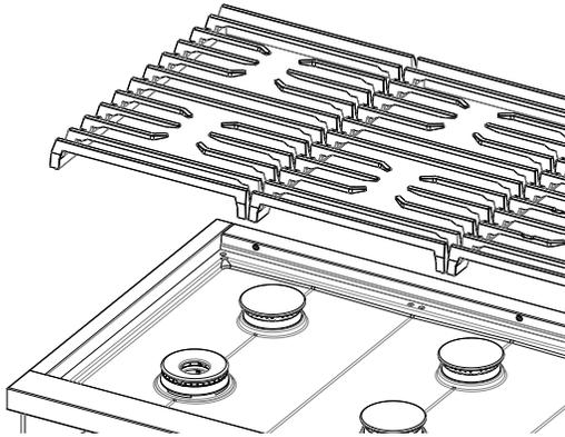
1. Remove the grates, then remove the burner caps and burner heads.
