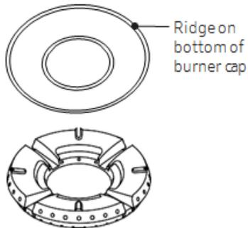
3. Put the burner caps on the burner rings. The ridge around the bottom edge of the cap fits around the top of the ring.
