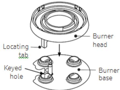
1. Place the burner heads as shown. The locator tab on the head goes in the keyed hole as shown.
