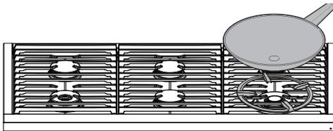
1. With all rangetop surfaces cool, place the wok ring on the grate on the 22K BTU Dual burner.
