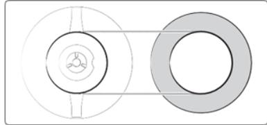
1. Orient the burner head so the electrode opening aligns with the electrode itself.
