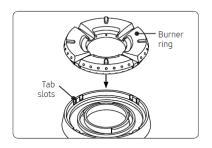
2. Put the burner rings on the heads as shown. Match the tabs on the bottom of the ring to the slots on the head. Wiggle each ring to ensure it is properly seated.
