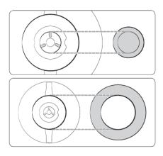
3. Size the burner caps to the burners, then install the caps on the heads.
