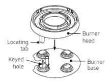
1. Place the burner heads as shown. The locater tab on the head goes in the keyed hole as shown.
