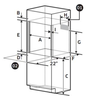
CABINET FLUSH DIMENSION А MIN. 30 1/4" (MIN. 76.7CM) В MIN. 1 3/8" (3.5CM) С MIN. 31" (MIN 78.7CM) D MIN. 2 1/2" (MIN. 6.4CM) Е MIN. 29 1/8" (MIN. 74.0CM) F MIN. 24 7/8" (MIN 63CM) G MIN. 22" (MIN. 55.9CM) Н MAX. 9 1/2" (MAX 24.1CM) - JUNCTION BOX MIN. 11/16" (1.75CM) - WOODEN CABINET THICKNESS L
