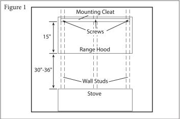
3. Rest the hood on the wood cleat with one person holding the hood. Score the drywall through at least 2 of the 3 holes located on the rear panel of the hood for placement of screws and/or drywall and anchors. Remove the hood and drill pilot holes into the marks transferred on the wall and add anchors if there is no stud(s) available.
