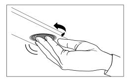
This range hood requires LED bulbs. (1.4W maximum per bulb) To change the light bulb, remove light case from the light socket. The light case can be accessed from the inside of the body of the machine.
