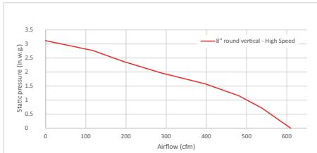
HVI-2100 CERTIFIED RATINGS comply with new testing technologies and procedures prescribed by the Home Ventilating Institute, for off-the-shelf products, as they are available to consumers. Product performance is rated at 0.1 and 0.25 in. static pressure at high speed based on tests conducted in an HVI-approved state-of-the-art test laboratory. Sones are a measure of humanly-perceived loudness, based on laboratory measurements.
