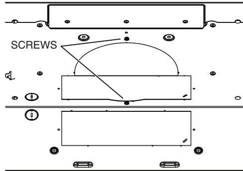
6 ] Remove Electrical Power Cable Knockout from top (vertical wiring) or back (horizontal wiring) of hood. Install an appropriate strain relief, 1/2" diameter (not included).
