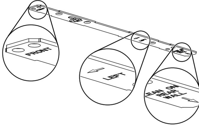
Refer to the marking on brackets to determine the correct installation side and orientation.
