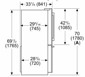
A: Add 1/4" (6 mm) with front leveling feet fully extended
