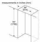
Leave ½" (12.7) gap at the top and 1" (25.4) behind the refrigerator for proper ventilation.
