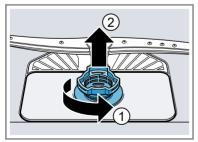
**3.** Pull the micro filter downward and off.
