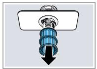
4. Press the locking catches ① together and take the coarse filter upward and out ②.
