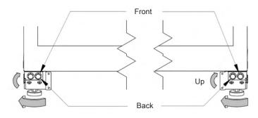
**Important**: Do not use a power drill and do not over-tighten the leveling bolts.
