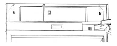
**Important**: If the mounting holes do not align with the slots in the top of the cabinet behind the top grille, it may be necessary to roll the refrigerator out of the enclosure, loosen the anchor bracket screws on the back wall, slide the bracket left or right, and retighten the screws.
