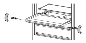
• **Replace**: Extend the slides. Align the tray on the slides and push back until the tray engages the rear hooks on the slides. Replace the Phillips screws on both sides of the tray (near the front). Do not over-tighten the screws. Set the glass on top of the tray.
