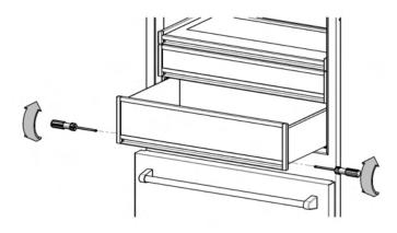
• **Replace**: Extend the slides. Align the drawer on the slides and push back until the drawer engages the rear hooks on the slides. Replace the Phillips screws on both sides of the drawer (near the front). Do not over-tighten the screws.
