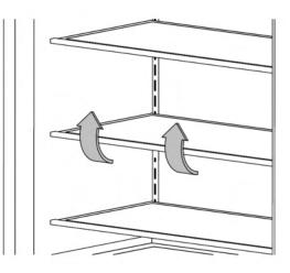
• **Replace**: Guide the rear shelf hooks into the shelf supports. Tilt the front of the shelf up until the rear shelf hooks drop in the shelf supports. Lower the front of the shelf and check to make sure that the shelf is securely in position.
