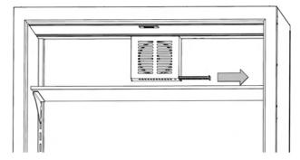
• **Replace**: Remove the air filter from the packaging. Align the air filter with the opening and slide it into the fan cover.
