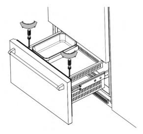
Replace: Extend the slides. Align the drawer on the slides and push back until the drawer engages the rear hooks on the slides. Replace the Phillips screws on both sides of the drawer (near the front). Do not over-tighten the screws.
