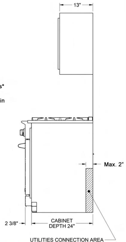
\* For non-ventilation installations clearance to combustibles BSDF36 & 48 is 40" min
