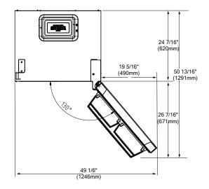
Required Minimum Clearances: Top: 2" Sides: <sup>1</sup>/2" on each side Back: 1 <sup>3</sup>/<sub>16</sub>"
