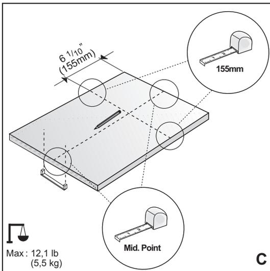
3. Mark the wooden door as shown in the drawing (Figure C).
