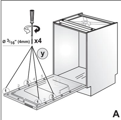
8. Using the four screws  $\text{Ø } \frac{3}{16}'' \times 1\frac{11}{16}''$  ( $\text{Ø } 4\text{mm} \times 43\text{mm}$ ) provided, attach the wooden door to the dishwasher at position 1 and 3 (Figure A).
