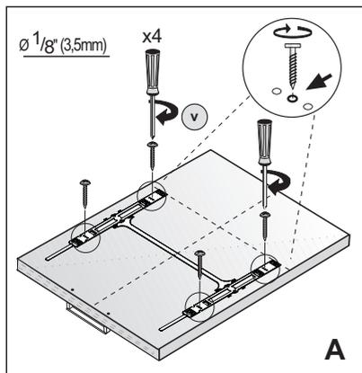
5. Attach the two mounting brackets to the wooden door with 4 screws ( $\varnothing 1/8"$  x  $5/8"$  ( $\varnothing 3.5\text{mm}$  x 14mm) (Figure A).
