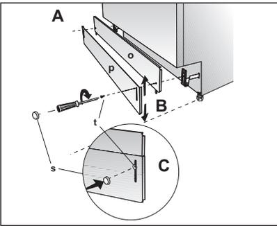
If the enclosure height is above  $33\frac{1}{16}"$  (840mm) use "o" and "p" labelled toe kicks together. Make sure the slotted toe kick "p" is on the outside so you can adjust height of the toe kick. Installation should be done following the steps illustrated in the figures A, B and C respectively.
