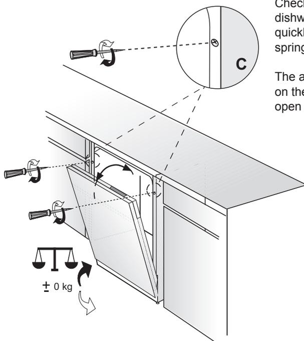
Check the door tension of the dishwasher: If the door closes too quickly or if the door falls open, the spring tension needs to be adjusted.
