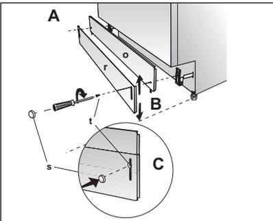
If the enclosure height is above  $34\frac{1}{4}"$  (870mm) use "o" and "r" labelled toe kicks together. Make sure the slotted toe kick "r" is on the outside so you can adjust height of the toe kick. Installation should be done following the steps illustrated in the figures A, B and C respectively.
