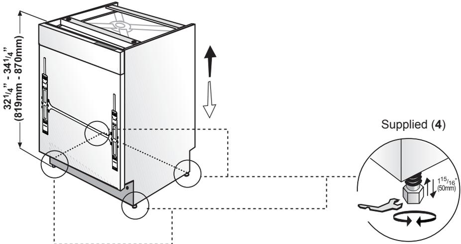
If the height of the enclosure is 33 <sup>7</sup>/<sub>16</sub>" to 34 <sup>1</sup>/<sub>4</sub>" (850mm - 870mm) use short supports as shown in the figure.
