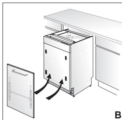
6. Mount the wooden door onto the dishwasher with the plastic mounting brackets which you have attached (Figure B).
