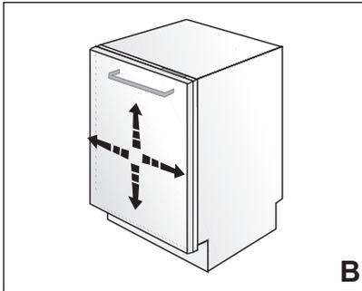
9. Check the position of the wooden door and make sure it is aligned properly (Figure B).
