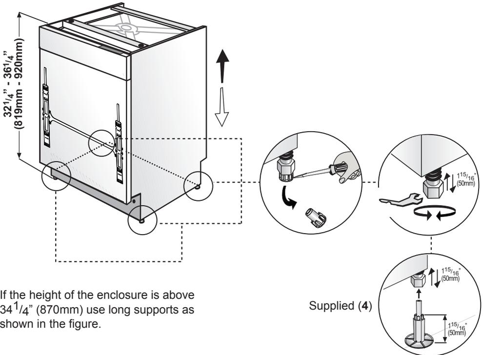
If the height of the enclosure is above 34 <sup>1</sup>/<sub>4</sub>" (870mm) use long supports as shown in the figure.
