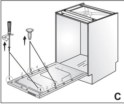
7. Open the door and remove the two caps and two screws inside the door at position 1 and 3 (Figure C).
