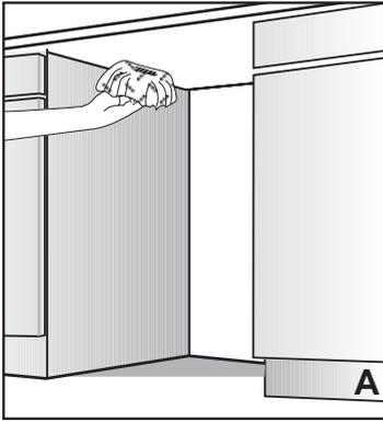
The steam protection foil will be applied at the location where the hot steam escapes when you first open the door (as shown in Figure B).
