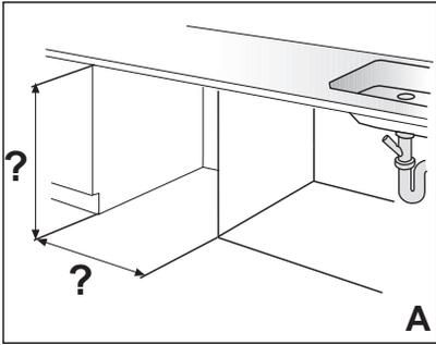
Measure the height and width of the enclosure (Figure A) and the toe kick. Determine how big the wooden door can be. For example if the height is  $33\frac{7}{8}$ " (860mm) and if the toe kick is  $3\frac{15}{16}$ " (100mm) the door can not be taller than  $29\frac{15}{16}$ " (760mm).
