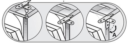
Place the two mounting brackets into the top corners of the dishwasher.
