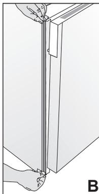
Place the trim strips on the front edge of the side walls (Figure B).
