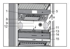
The serving area (zone B) is a temperature zone between the top (5) and bottom (15) insulation barrier. It allows you to bring the wine on ideal consumption temperature, and to prepare in advance everything you need for quick and top-notch wine serving: chilled wine glasses, space for already open bottles, decanter, and other accessories (bottle openers, wine pourers/spouts, stoppers ...).
