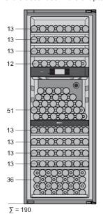
Up to 51 Bordeaux bottles can be loaded onto the bottom insulation barrier.
