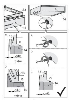
If the shelf (13) and drawer (14) are not aligned at the front (d≠0), first completely pull out the drawer to access the drawer opening mechanism on the back wall. Press on the spacer (A) to release the mechanism. Rotate the spacer to adjust the length.
