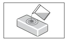
Fill the box with 0.5 litre of tap water and place it in the relevant zone. There are no preferrable positions, as long as it is placed in the correct zone.
