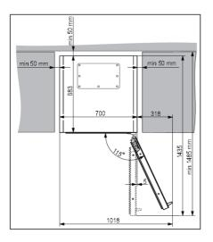
To allow for adequate ventilation and cooling of the appliance, there has to be sufficient clearence behind the appliance and on both sides as well (at least 50 mm). Please, also observe the clearance required to fully open the door in order to allow pulling out the drawers and shelves (see installation diagram).
