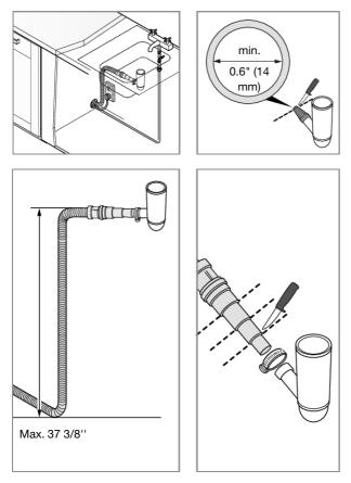
The drain hose can also be connected to a connection nipple on the sink unit's water trap. The connection nipple must have an internal diameter of at least 1/2".
