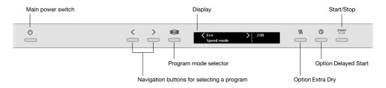
Install the dishwasher, see the chapter *Installation instructions*. Following this, open the door and press the main power switch to start using the machine.
