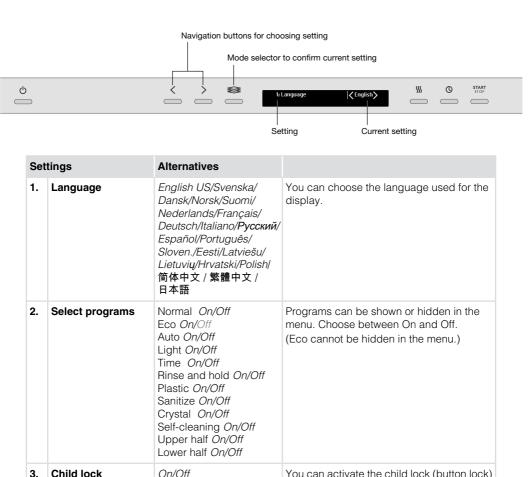
the child lock, press and hold the left Navigation button and the option button Delayed Start for 3 seconds.
