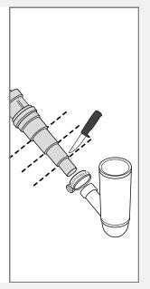
The drain hose can also be connected to a connection nipple on the sink unit's water trap. The connection nipple must have an internal diameter of at least 1/2".
