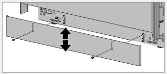
Ensure the floor underneath the toe kick is at same height as the floor underneath the dishwasher.
