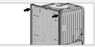
If a height of 32  $1/4^{\prime\prime}$  is required, remove the upper trim kit. Also lower the trim kit on the sides.
