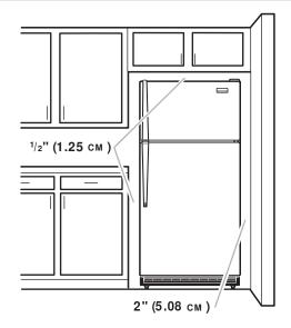
To ensure proper ventilation for your refrigerator, allow for a  $\frac{1}{2}$ " (1.25 cm) space on each and between overhead cabinets and refrigerator top. Allow at least 1" (2.5 cm) between back of cabinet and the wall. If your refrigerator has an ice maker, make sure you leave some extra space at the back for the water line connections.
