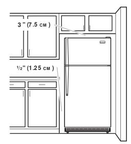
To ensure proper ventilation for your refrigerator, allow for a %" (1.25 cm) space on each side. Allow 3" (7.5 cm) of space between overhead cabinets and refrigerator top. Allow at least 1" (25.40 mm) between back of cabinet and the wall. If your refrigerator has an ice maker, make sure you leave some extra space at the back for the water line connections.
