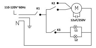
protection thermique L1 L2-Lamp M-Motor K2-Motor Switch thermally protected K1-Mains Power Switch K3-Lamp Switch
