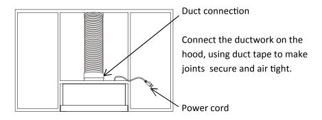
Your new range hood will operate at the highest efficiency if the number of elbows and the length of the duct are kept to a max of 15ft. (Note 1 x elbow=4ft)
