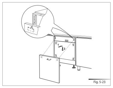
Secure the door to the panel with the supplied screws. The panel must have a minimum thickness of 20 mm (25/32") (see fig. 5-24).
