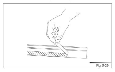
Fix the gasket to the dishwasher, inserting it in the seat on the sides towards the front (see fig. 5-30), and making sure that the long side of the gasket, the one with the hole for inserting the screw, is attached to the outside of the dishwasher; the hole in the long side must match the hole in the dishwasher (see ref. A fig. 5-31). Make sure the gasket adheres perfectly to the dishwasher.
