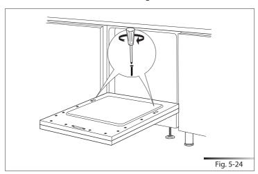
Make sure the dishwasher door, complete with panel, opens comfortably and that the base plate (ref. A fig. 5-25) does not prevent it from opening fully. If the base plate prevents the door from opening, mark out the section to remove (see fig. 5-25), take out the base plate and cut it along the marking using a compass saw (see fig. 5-26).
