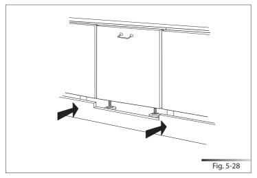
Before securing the dishwasher to the adjacent units, attach the gaskets to the sides.
