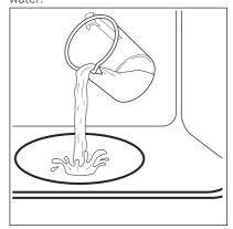
The maximum capacity of the cavity embossment is 250 ml. Fill the cavity embossment with water only when the oven is cold.
