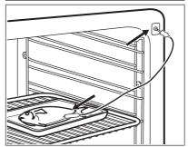
The display shows the core temperature sensor symbol.
